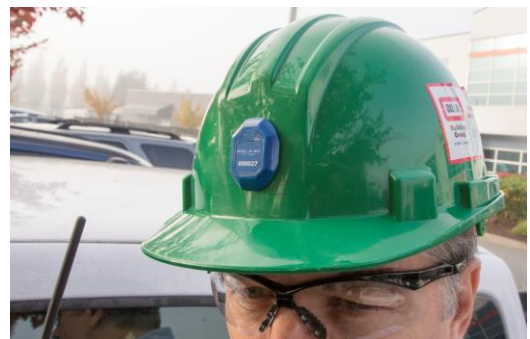
A GuardRFID AT-4 active tag is being attached to each worker's hardhat
